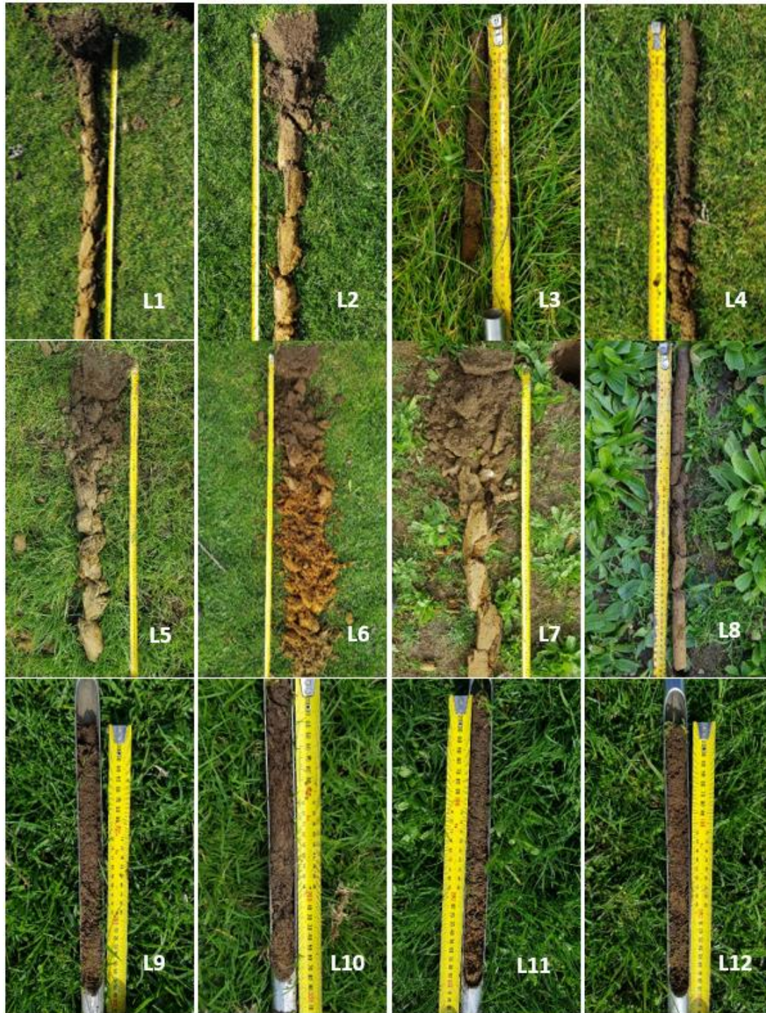
Figure 3: Examples of topsoil and subsoil depths (left to right and top to bottom) from sampling locations L1-L12 (refer blue numbers in Figure 2).
